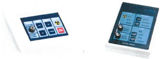
Remote text displays at the console area and on the afterloader itself provide information on the source position and status.
