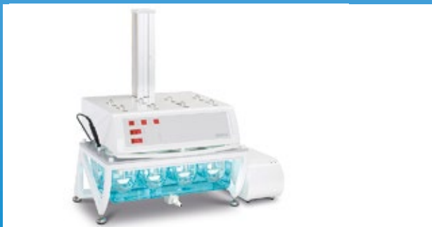
DT 728 in Low-Head mode to minimise evaporation
