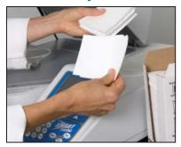
CEM sample pads were specifically developed for use in our microwave moisture and fat analyzers to assure the accuracy demanded for process and quality control. The pads are manufactured to meet our strict requirements for absorbance, moisture content, and strength for consistent results. They are approved for use with AOAC Official Methods and are manufactured at our ISO-approved facility.
