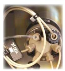
Exchangeable Sample Loop made of PEFK
