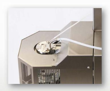
On-line connection from GPC directly into the EVAporation chamber - possibility of precise concentration up to 0.2 mL.
