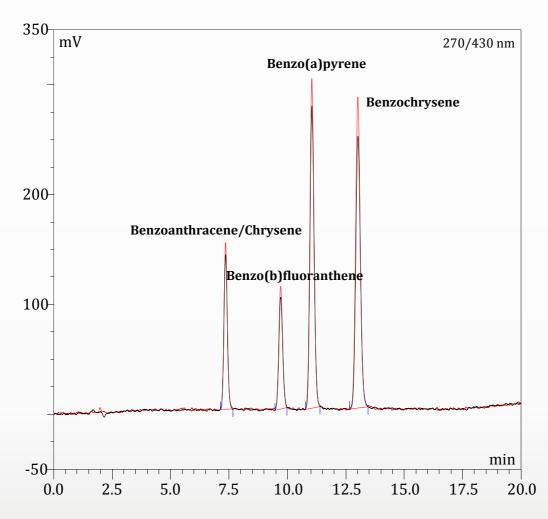
The figure shows the overlay of two fluorescence chromatograms: external PAH standard (red) and a finished sample (black).
