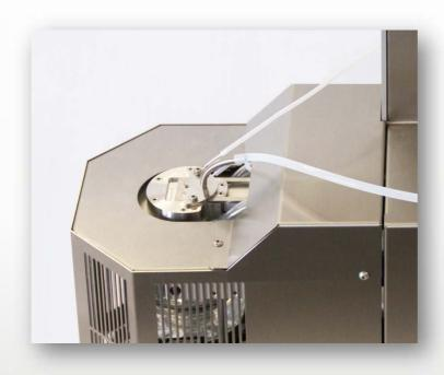
On-line connection from GPC directly into the EVAporation chamber – possibility of precise concentration up to 0.2 mL.
